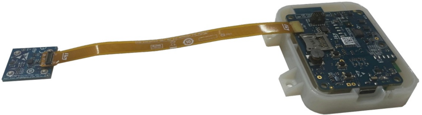
Figure 3. Plugging the flexible cable onto the STWIN. box
