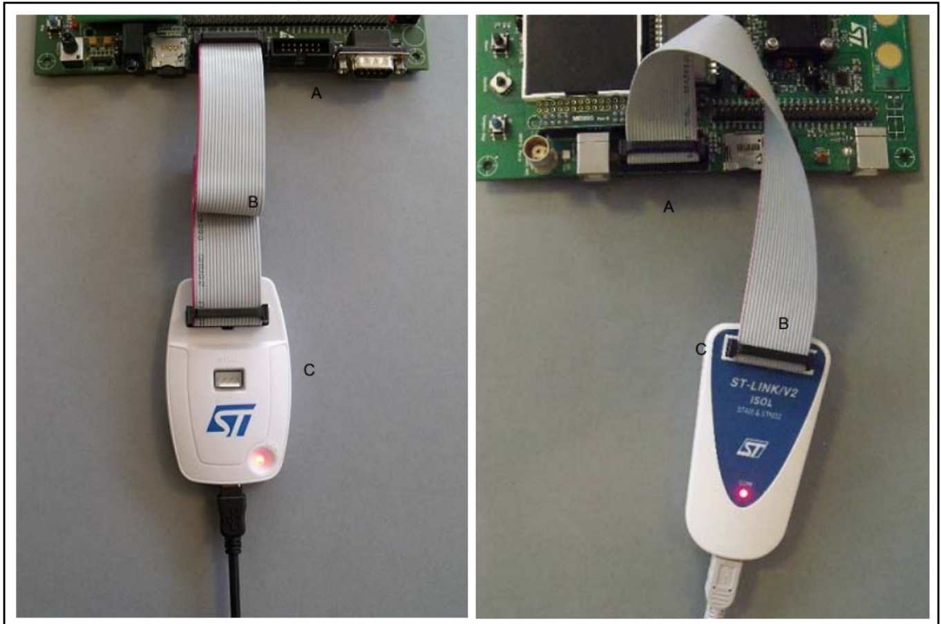
Figure 9. JTAG and SWD connection
