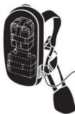
Carrying system with built-in “AP belt bag with connecting cable” together with the support cushion
