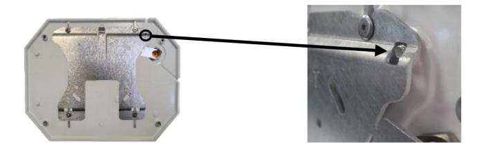
Step 2: Unscrew the locking screw with Torx T8 tool, without removing the screw from the plate so as not to lose the seal.
