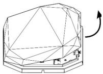
The reader is equipped with a locking screw that secures the reader plate to the metal mounting plate.
