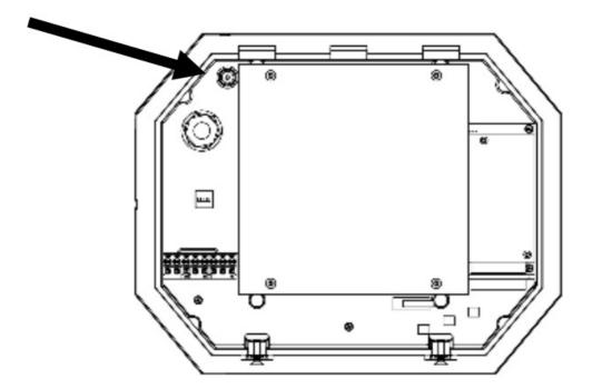
**Step 3:** Remove the metal mounting plate by exerting pressure on the metal plate while sliding it. Leave the four mounting screws in place.
