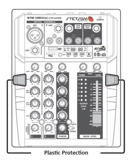
• Choose a place with easy access to install the product. When necessary to attach the product, use the holes that are protected by plastic. Remove the plastic protection and fasten with screws.
