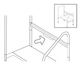
Peel two-sided tape off back of light (G) and attach to light bracket on part C with light & sensor facing out. See other side for details.
