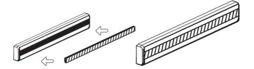
Attach magnet side (front) of double-sided tape to the magnet side of the light.
