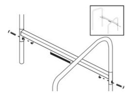
Insert two bolts (F) then apply & tighten nuts.
