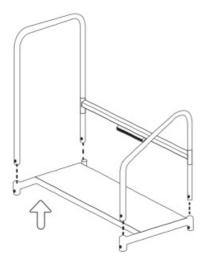
Insert A & B into holes of part D and raise to align with bolt holes.
