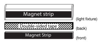
Locate light with magnet strip and double-sided tape.
