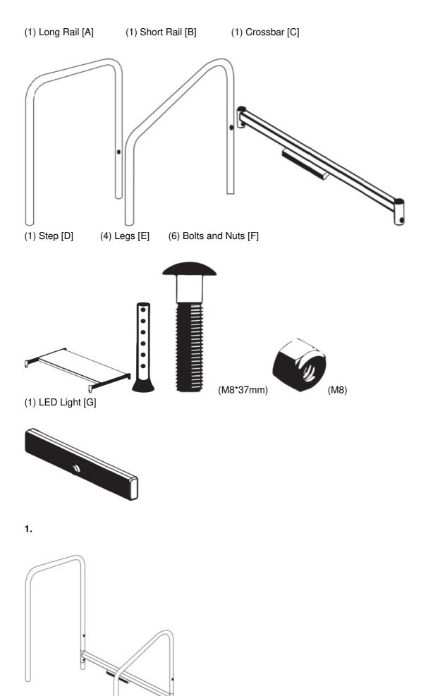
Insert A & B into holes of part C
