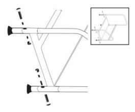
Insert four bolts (F) then apply & tighten nuts.
