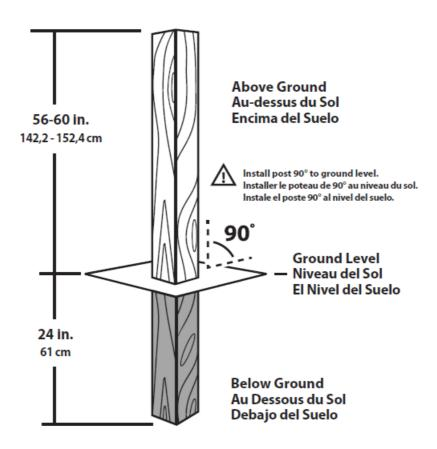
Check that post is straight and firmly secured in ground. Post must be 56-60 in. (142.2-152.4 cm) from ground.
