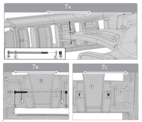
Repeat process to other end of brace (X). Tighten bolt (A) and nut (B) using rachet and wrench.
