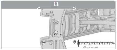
Using screw (M), connect base (AA) to steps (Y).
