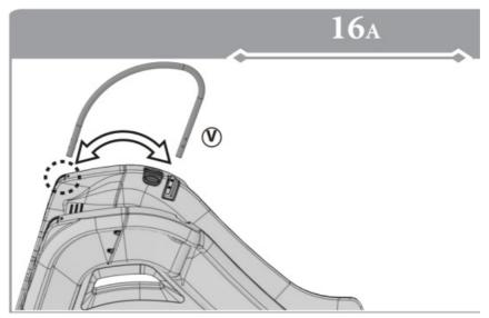
One person should get on top of the slide to help apply pressure. Start with getting the back of the handle in first. The other person should help line up the front part of the handle.
