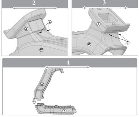
Lay down steps (Y) and lower in slide (W) applying downward pressure to help close gaps.
