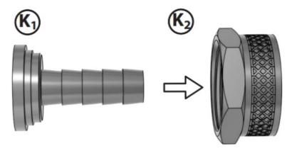
Using soapy water attach hose attachment (K) to hose (T) until fully inserted and secure.
