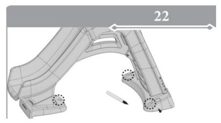
Once holes are marked, move slide and use included drill bit to drill into concrete for anchor installation.
