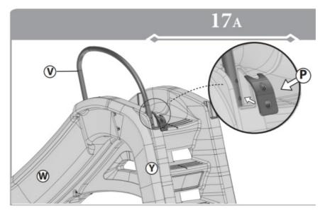
Start by placing handle bar (V) in and lining up back holes with plate (P) for bolt installation.
