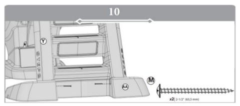
Stand slide upright for installation of the screws into the base of the steps. This will help prevent gapping.
