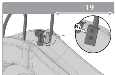
Line up the holes on the plate(N1) with handle (V) and install bolts (C) making sure plate is flush. Repeat process to other side.
