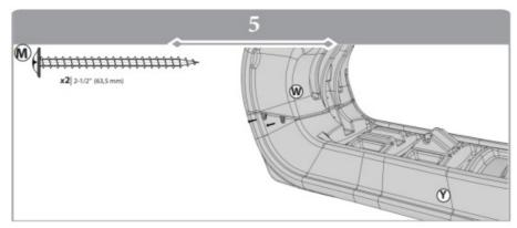
Person 2 should be applying pressure to minimize gaps. Person one should be installing screws (M). Repeat to other side.
