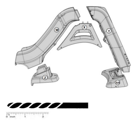
Measure 2 in on drill bit (R) and mark it for later use.
