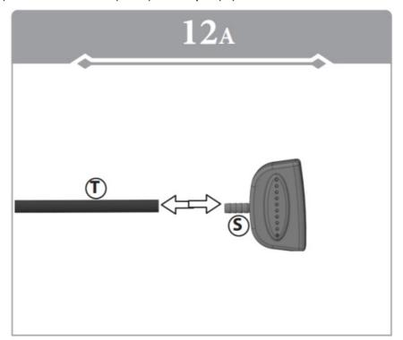
Use soapy water to attach sprinkler head (S) to hose (T) until fully secured.
