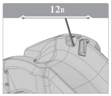
Feed hose (T) through slide till sprinkler head (S) is in place.
