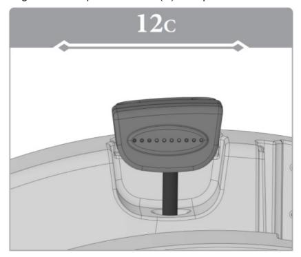
Make sure when inserting tube (T) through slide, that Sprinkler head (S) lines up creating no gaps.
