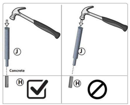
Once holes are drilled using provided masonry drill bit (S) to a minimum depth of 2 inches, use a hammer on the anchor tool (J) to drive anchor (H) into concrete. Making sure top is flush when complete.
