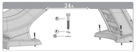
Using a 3/4" socket, attach bolt (E), lock washer (F), and flat washer (G) to anchor (H). Tighten till secured.
