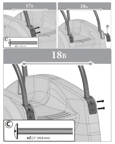
Once both handles have been bolted into the steps and secured, the person putting bolts in should line up the holes for bolt install. The second person needs to hold handle in place and apply downward pressure.
