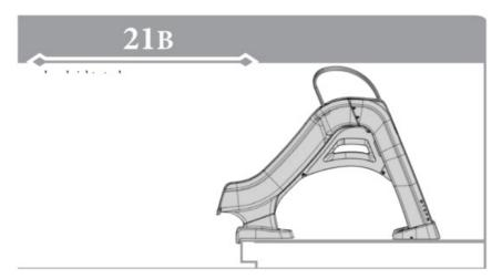
**NOTE:** Slide needs to be set with overhang placed right at edge of concrete for proper anchor installation.
