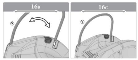
While holes are lined up have one person holding Handle in place while other attached bolts.
