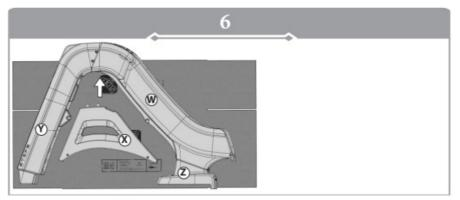
Using 2 people, attach support brace (X) into steps (Y) and slide (W).
