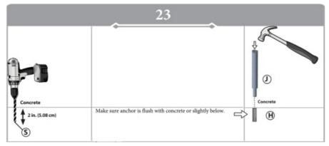
For drilling and anchor installation hole needs to be drilled straight otherwise installation will not hold slide in place.
