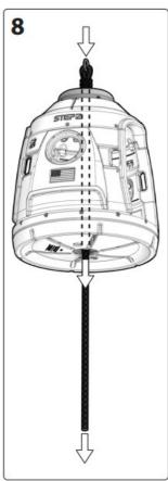
Remove Knot Tying Template & Guide (Next page KT1-KT4) from this instruction sheet. Use Scale template to mark rope to ensure correct rope knot with a minimum 4" tail.
