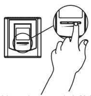
The minimum set point is 3°C (37°F), and the maximum set point is 30°C (86°F). In Day mode, you can turn off the thermostat by lowering the set point below 3°C. The set point value displayed
