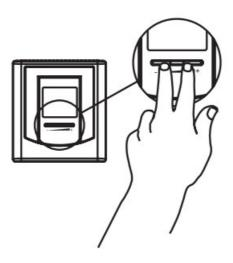
The current Day/Night mode selection is indicated on the display by the Sun or Moon icon. In order to manually switch from one mode to the other, simultaneously press down the two buttons and release them immediately.
