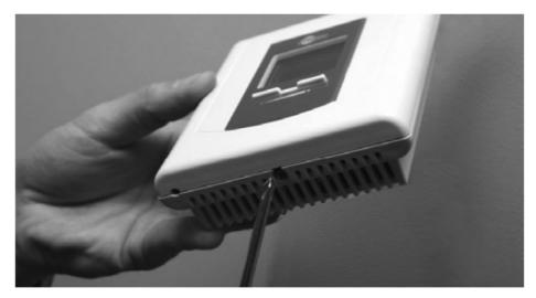
5. Align and secure the mounting base to the connection box using the two screws supplied.
