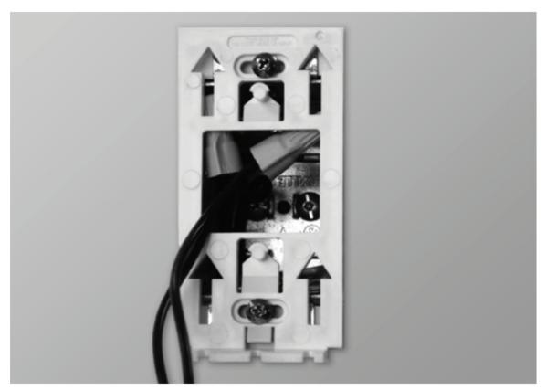
7. Align the little slots located on the top of the thermostat with those on the mounting base and secure the thermostat to the mounting base. Note that you can also position the thermostat on the left or right side of the junction box (see the illustrations below). Then, tighten the screw at the bottom of the unit.
