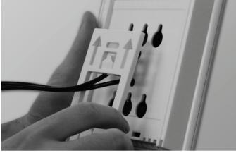
Then, remove the mounting base at the back of the thermostat by tilting it downward, then towards you.
