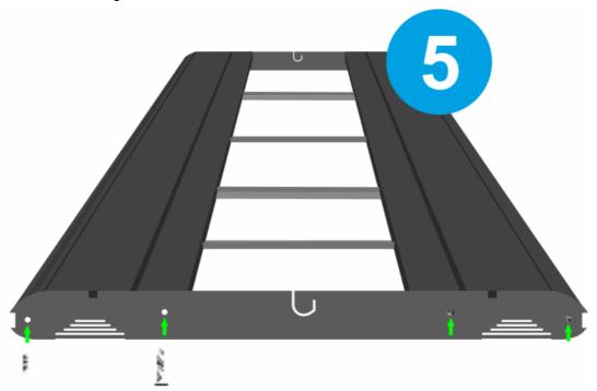
Now slide the mounting brackets or your LED fixture in the desired position or add another pair of mounting brackets for additional LED fixtures.
