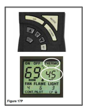
To exit THERMO mode press the MODE button. This also shuts fireplace OFF.
