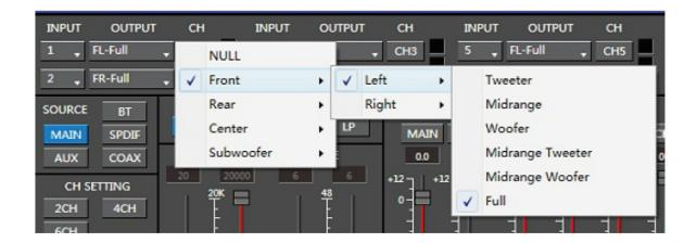
Options on the Link are for combining settings for Left CH and Right CH. Options on the Left CH/right CH allow you to tone each selected channel respectively
