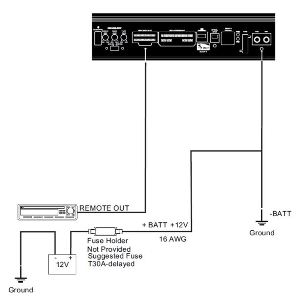
**Remark:** the DSP is internally protected by a Fuse-resistor soldered on its printed circuit board To replace it contact a service center. Using an External fuse is recommended, though it is not required.
