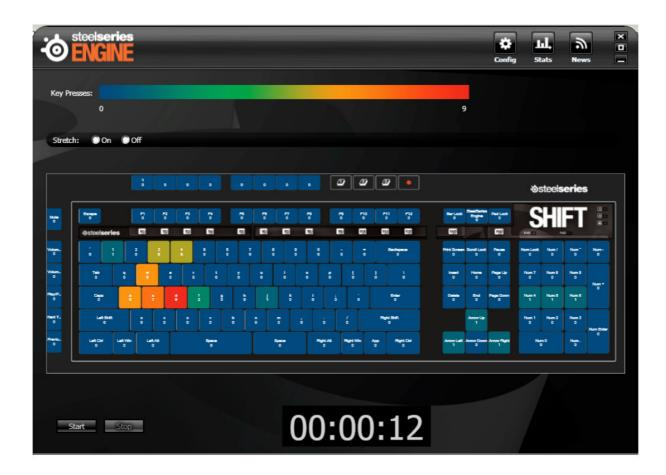
The color coding will help indicate which keys were pressed more often, and the entire test will be timed. Keep in mind that while running the test, every key on the keyboard will still be active.
