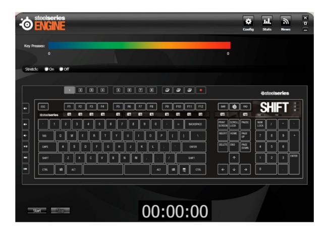
To use it, press the Start button near the bottom of the window, and press the keys on your keyboard at your discretion. Press the Stop button at any time to stop the test, and the display will output how many times each key was pressed.
