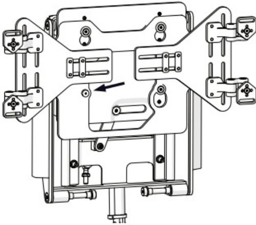
**Step Two:** Slip the adapter plate over the knobs and press it into position. Replace the thumb screw in the lower left hole of the adapter, as shown.
