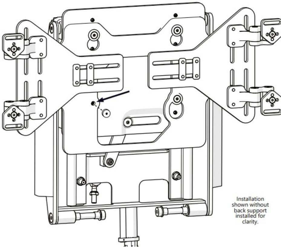
**Step Eight: Install the Thumb Screw:** The thumb screw is designed to hold Adapter Plate (B), and the back support attached to it, securely to the spine of the chair. Do not attempt to operate the chair without installing the thumb screw into the location shown in the image above.
