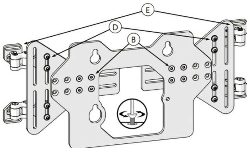
**Step Two – Adjust the Width:** Adjust the Adapter Wings (B) to the approximate width of the slots in the back shell. The four flat head screws that secure the Adapter Wings (B) to the Adapter Plate (A) can be installed in three different mounting positions to accommodate an extra two inches (2") in width. Choose the best position and snug the flat head screws to secure the Adapter Wings (B) in position. See "*Adjustment – Mounting Plate Width Adjustment*".
