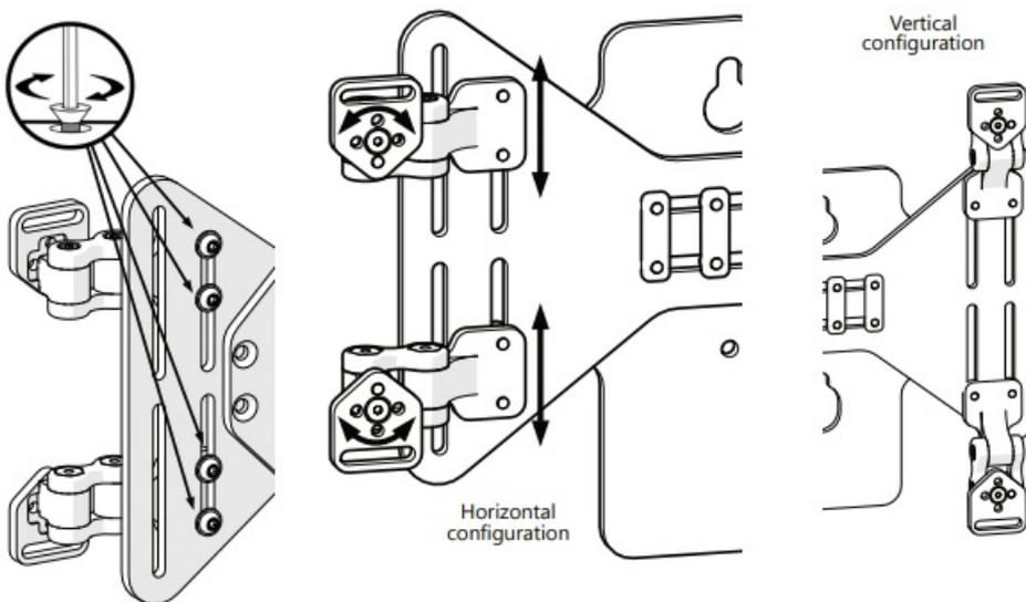
**Step Four – Mounting Plate Rotation:** If necessary, loosen the flat head screws and rotate the Mounting Plates (E) to properly orient the slots in the Mounting Plates (E) with the mounting locations of the back support. See *Adjustment – Mounting Plate Rotation*.
