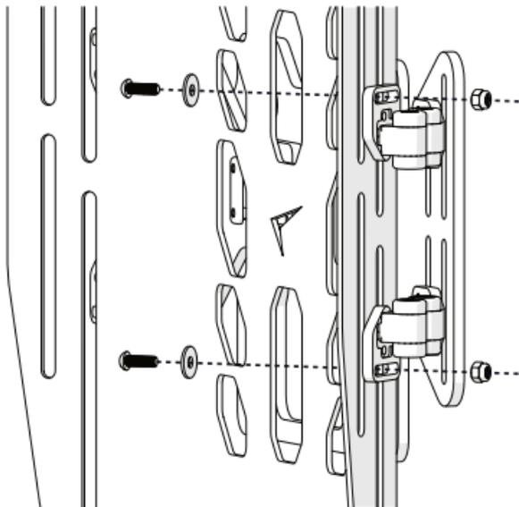
**Step Seven – Install Adapter Plate to the Chair:** Align the mounting locations on the Adapter Plate (A) with the mounting posts on the chair back. Slide the Adapter plate over the posts and it should slide into position on the posts.
