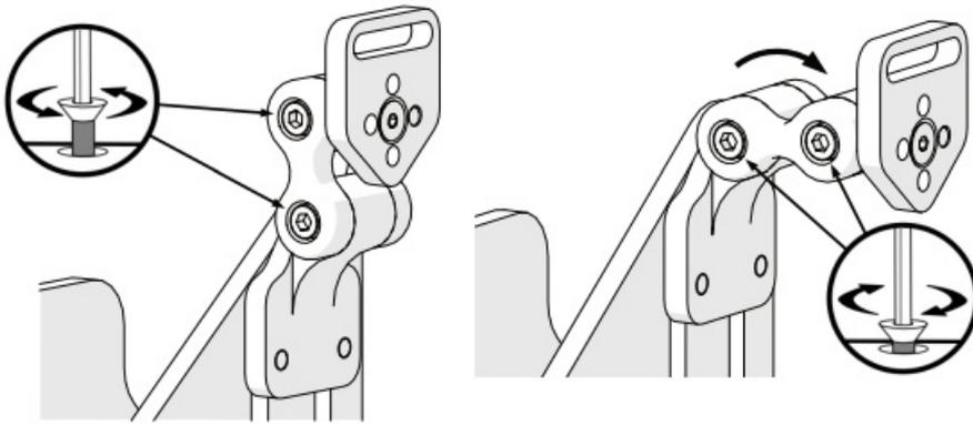
**Step Six – Attach the Shell:** Insert the button head screws through the fender washers and the front (user) side of the back support and attach to the Mounting Plates (E) using nylon lock nuts.
