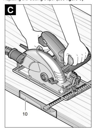
Adjust the cutting depth to the thickness of the workpiece. Less than a full tooth of the blade teeth should be visible below the workpiece.
