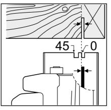
The 0° cutting mark 9 indicates the position of the saw blade for right-angled cuts. The 45° cutting mark 8 indicates the position of the saw blade for 45° cuts. For precise cuts, position the circular saw against the workpiece as shown in the figure. It is best to carry out a trial cut.
