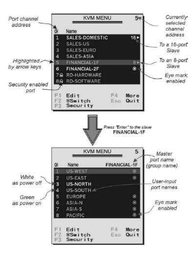
By hitting the left <CTRL> key twice within two seconds, you may see the 'Hotkey Menu' if it is enabled (an OSD option). Or, by hitting the left <CTRL> key three times within two seconds, you will see a 'KVM MENU' screen showing a list of the computers with corresponding channel addresses, names and status. The channel address (port number) of the currently selected computer is displayed in red, same as the front indicator, to the right of the OSD title 'KVM MENU'.
