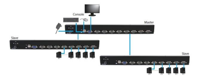
NOTE! A device (computer or KVM switch) at any 'PC x' port can be changed at any time after initial power-up. If you change any one of the PC 1 to PC 8 port connections from a computer to a Slave KVM switch or vice versa, or replace the devices of a port, the OSD will update this change the next time it is activated.
