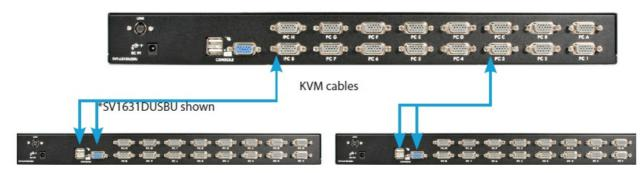
The maximum number of computers controlled by a Master/Slave configuration with all 8-port KVM switches used is 64, with 8 Slaves and each Slave connecting to 8 computers: The maximum number of computers controlled in a Master/Slave configuration with all 16-port KVM switches used is 136, with 8 units of 16-port Slaves (to PC 1 – PC 8) and each Slave connected to 16 computers, plus 8 more computers connected directly to the Master (to ports PC A – PC H):
