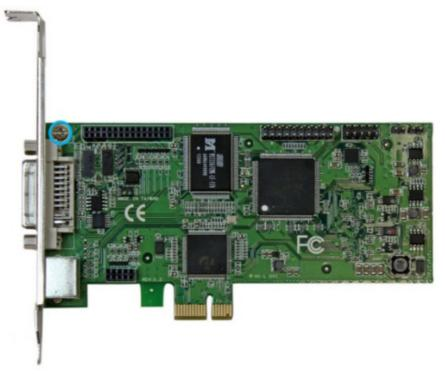
3. You can now remove the undesired bracket by pulling the bracket away from the capture card.
