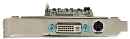
2. Using a Philips-type screwdriver (not included), remove the screw located next to the internal side of the DVI port on the circuit board.
