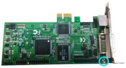
6. Re-insert the Standoff screws that you removed in step 1.
