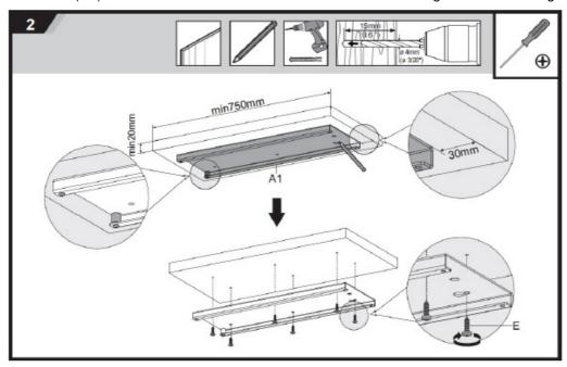
Slide the Arm Assembly (B) into the Guide Track (A1)
