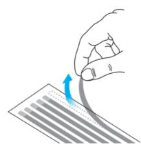
4. Carefully align the Adhesive Strips along the Top, Bottom, Left, and Right edges of the Privacy Filter. Apply Firm Pressure to affix them to the Privacy Filter.
