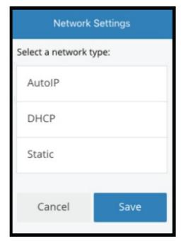
6. Using the on-screen keyboard, enter an IP address and subnet mask for the device. – or – Select DHCP and your network will automatically assign an IP address and subnet mask to the device in the range of the rest of your network devices.
