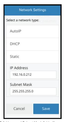
5. Select the Static button, and an IP Address and Subnet Mask field will appear.
