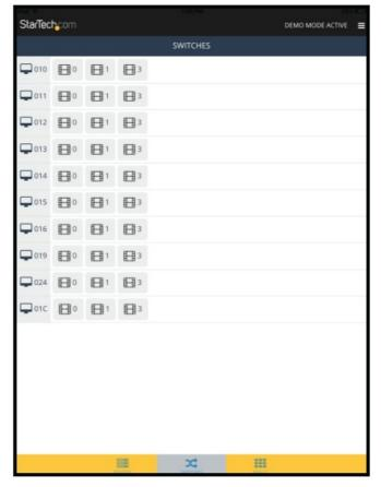
3. A list of connected receivers and transmitters will be displayed. The transmitter that is currently selected for each receiver will be highlighted in yellow.
