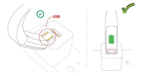
USB is a single-face device, and you may notice there is only one face with a metal piece, if you plug it in a reversed way, the fitness tracker will not receive power.
