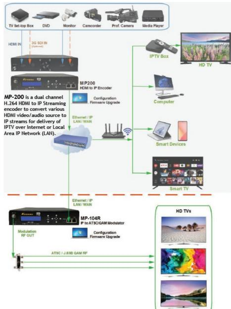
MP-104R is quad channel ATSC/J.83B QAM modulator to convert IP streams received from Internet or LAN IP network to ATSC / J.83B QAM RF signal for delivery of IPTV over coax network. IP Streaming to ATSC/J.83B QAM RF Output
