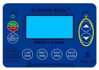
• Press the SET/RESET button to step over from hours to minutes and from Start Time to Stop time
