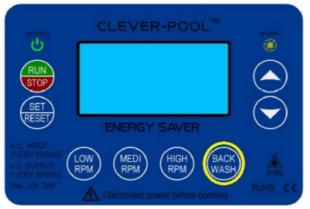
• Press the BACKWASH button. The display will now show backwash and the rpm.
