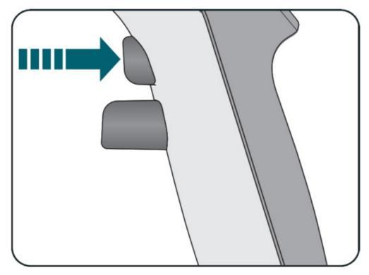
To quickly aspirate or dispense liquid, press the corresponding control button firmly.
