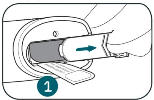
2. Remove the battery and discharge protection.
