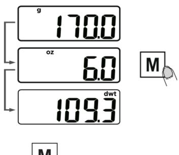
• Press button to switch the weight measure.
