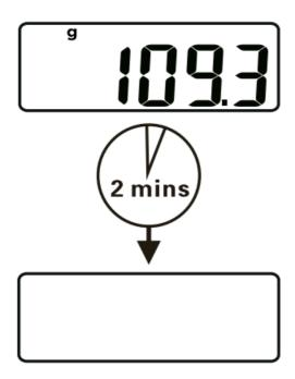
Auto shut off occurs if display shows "0" or shows the same weight reading for 3 minutes.
