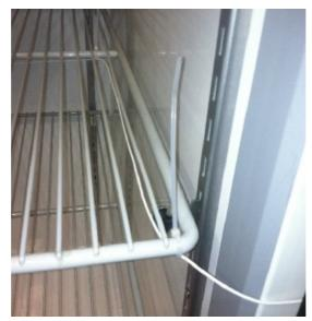
• Continue to route the cable towards front of the fridge/freezer on the hinge side and secure. If you have a cable port on your fridge/freezer you could route the cable through that.
