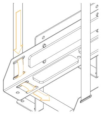
5. Loop the straps through the buckles as shown in these 4 steps. When tightening to your computer, have straps tight then push buckle closed which will tighten slightly further for a snug fit.
