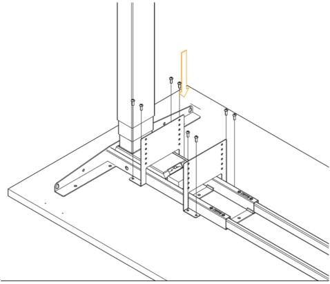
3. Once the brackets are screwed into position, its time to install the mount. Use the short machine screws to complete this step.
