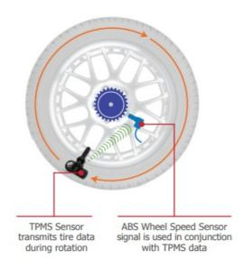
Auto-Relearn automatically identifes each TPMS sensor, determines its position on the vehicle, and then wirelessly transmits the information to the receiver for display on the dash – all without human intervention. For a better understanding, here are two popular Auto-Relearn technologies.
