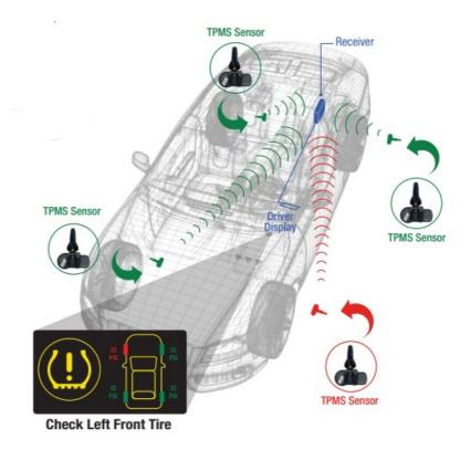
Wireless Auto-Locate systems use advanced TPMS technology along with RF signal strength to determine sensor location after installing a new sensor or tire rotation.
