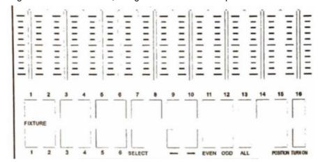
There are 6 pages of fixtures supporting up to 96 fixtures. The <Attribute/Level> button with 2 LED indicators can be used to switch the functions of the 16 sliders. When <Attribute> is activated, the sliders are used to adjust the value of the attribute above the sliders; When <Level> is activated, the sliders are to adjust the intensity of fixtures.
