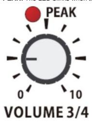
**VOLUME** This fader adjusts the final output level of the **MAIN** outputs for the Stereo channel only. To prevent noise, the fader should be set to 0 when the channel is unused. Ideally, the fader should be set close to 10 for maximum fade control. Adjust the **GAIN** of the input signal so that the **VOLUME** fader can be set to 10 without
