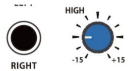
**HIGH:** Adjusts the amount of treble in the signal. The gain range is -15dB - +15dB, with a center frequency of 12kHz.
