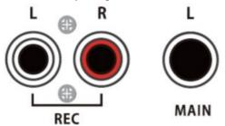
MAIN A stereo pair of unbalanced 1/4' TS outputs that serve as the primary mixed output
