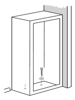
For optimal security, your safety must be mounted to the floor. The safe should be installed in a dry, secure area, adjacent to a sidewall and with minimal space on either side.
