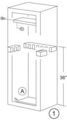
To install the barrel rests to the cabinet, first remove the backing from the foam rests. For help in doing this, pinch the end of the foam to help secure the adhesive to the foam. Attach the barrel rests to the inner sides of the cabinet as shown.
