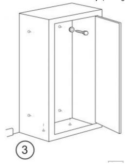
Drill (4) 3/16" pilot holes into the wall studs and secure the cabinet to the wall using (4 ea.) lag bolts and washers. (See figure 3)
