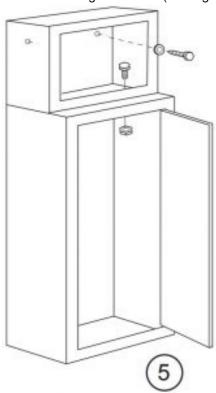
Drill (4) 3/16" pilot holes into the wall studs and secure the GC-500-5 cabinet to the wall using (2) lag bolts and washers. (See figure 5) Tighten the (2) bolts that connect the cabinets.
