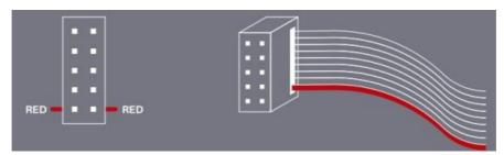
If you flip over your ST·FONT, you will find the "RED" mark at the PCB power connector, which must match the colored line on the ribbon cable.
