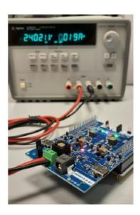
• any DC power supply that allows the board to provide up to 120W output power (60W on each port), must be connected to the DC Power Connector J801.
