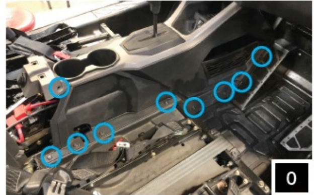
O. Remove the (1) push pin and (8) T40 screws from each side of the remainder of the center console.
