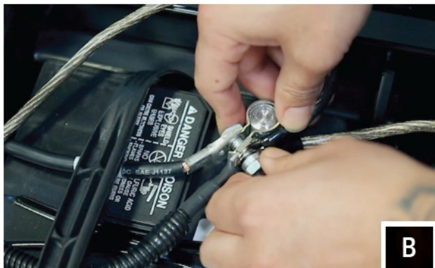
B. Unscrew the factory nut on the negative battery terminal. Install the 2 ground cables to the screw on the ground battery terminal. Re-install the factory nut.
