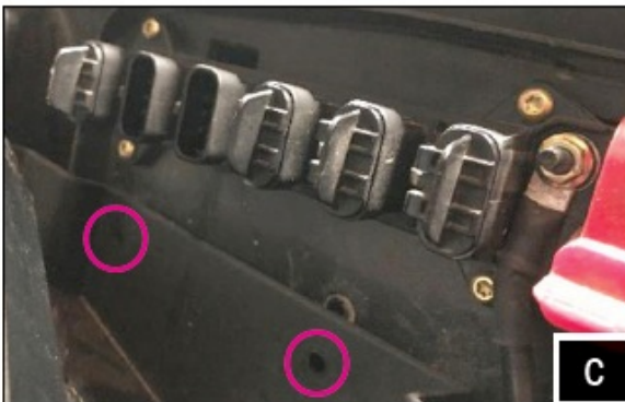
C. Extract (2) T25 screws located at the back of the plastic tray, once extracted remove the plastic tray.
