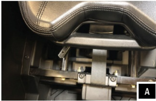
A. Remove all the seats from the vehicle. Compress the release lever located in front of the seat base. With the release lever compressed, tilt the seat forward and remove from the vehicle.
