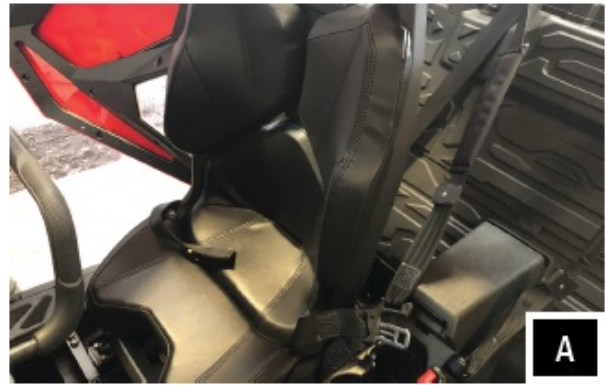
A. Remove all the seats from the vehicle. Compress the release lever located in front of the seat base. With the release lever compressed, tilt the seat forward and remove from the vehicle.
