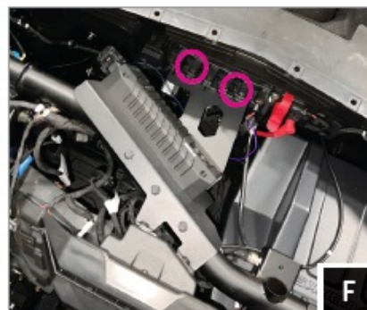
F. Replace the (2) T25 screws.
