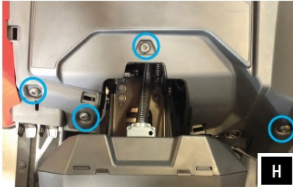
H. Remove the (4) T40 Torx screws that surround the gauge cluster. For ease of access to each screw we recommend adjusting the position of the steering column accordingly.
