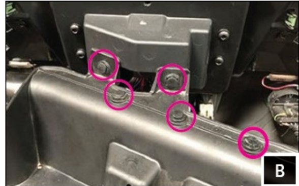
B. Remove the (5) push pins located on the plastic tray in the dash cavity.
