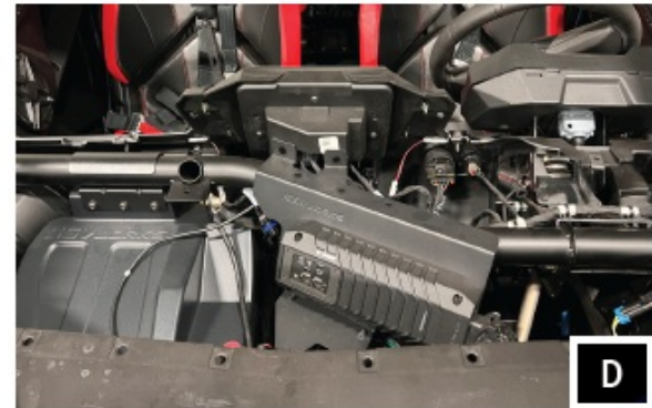
D. Line up the 800.5 amp plate in the same location.
