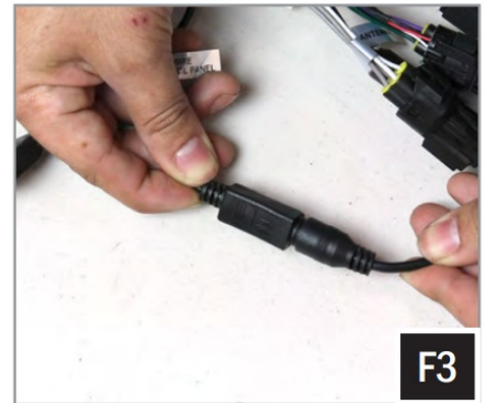
F3. Re-assemble dash and route controller cable into dash cavity and connect to MRB3 brain.
