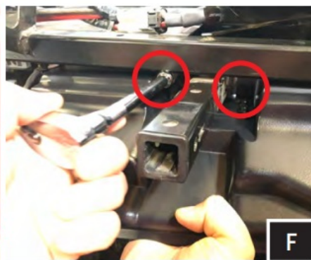
F. Lift the enclosure into place. Using the factory glove box mounting hardware, fasten the enclosure into place.
