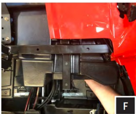
F. Lift the enclosure into place. Using the factory glove box mounting hardware, fasten the enclosure into place.
