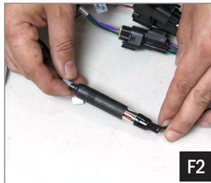
F2. Connect the antenna. Route the antenna wire under dash.
