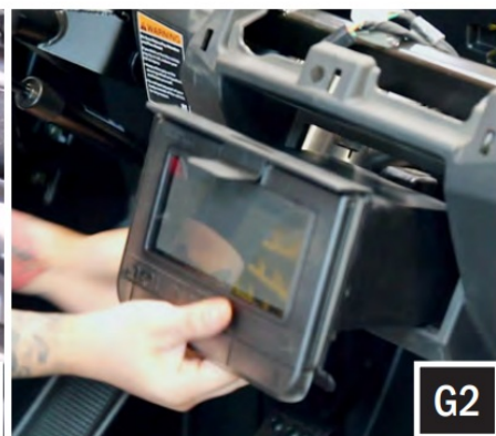
G. Remove the factory dash pocket by first extracting the 10mm bolt on the dash frame (G1). Then pull out the dash pocket with the bracket attached (G2) –
