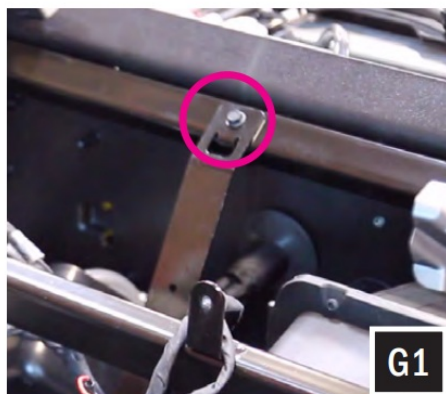
G. Remove the factory dash pocket by first extracting the 10mm bolt on the dash frame (G1). Then pull out the dash pocket with the bracket attached (G2) –
