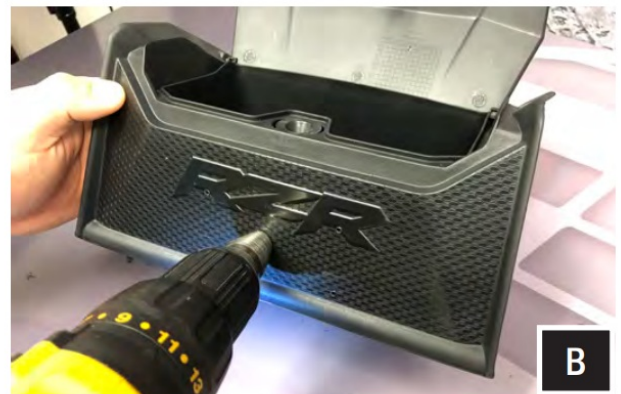
B. Remove template, drill out pilot hole with 1-1/8" drill bit
