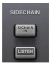
Hi- and Lo-pass filters are available for the Compressor side-chain. To switch the filters into the compressor side chain, switch the S/Chain in button on. To listen to the Compressor side-chain, click on the Listen button. Adjusting the filter controls will change the signal that triggers the gain reduction; removing low-end frequencies from the sidechain can reduce unwanted pumping effects, for example.
