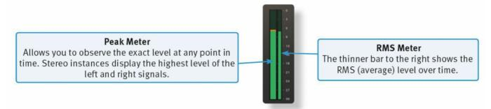
When clipping occurs, the meter will turn red. It will remain red until the meter is reset by clicking on the meter.
