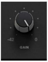
Turn the GAIN knob in the input section to control the level of the incoming audio signal. The post-gain signal level is shown above. Turn the GAIN knob in the output section to ensure that the signal retains a good signal level post-processing. The output signal level is shown above the knob.
