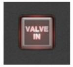
Valve in introduces a tube compressor emulation for saturating the signal by adding harmonics.
