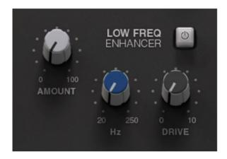
The HF and LF enhancers respectively enrich the high and low frequencies of the input signal. Whereas a standard EQ simply raises the level of certain frequencies, the Enhancer adds a combination of 2nd and 3rd harmonics to those frequencies, producing a more pleasing effect.
