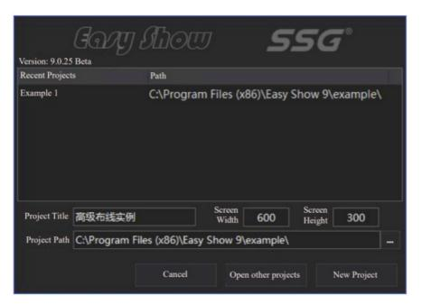
11. Click the New Project to pop up the new advanced layout message text box, and enter the name of the new layout file "advanced layout display screen\_1\_partition\_1";
