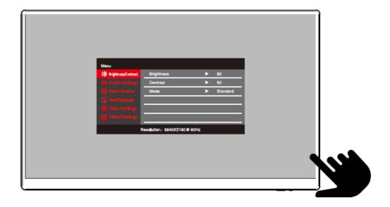
Short press the OSD menu for 3 seconds to activate it (the ▼menu will automatically exit after 8 seconds without any action),
