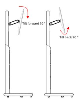
$\bullet\,$  The monitor can tilt forward 45  $^{\circ}$  and backward 20  $^{\circ}$
