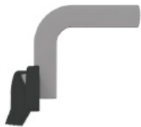
(1) Trub Dam Dip Tube
