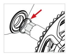
Due to tight tolerances, the axle/bottom bracket can be difficult to install if not inserted straight. Carefully align the spindle with both bearings and with a slight rocking motion use light pressure to fully seat crank in the bottom bracket. Make sure that the Non-Drive Side bottom bracket does not come loose or even come out of the BB shell.
