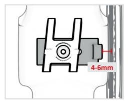
• Install the bolt and tighten it to the torque specified by the frame manufacturer – you may need a longer screw to securely hold the cable guide and magnet in place.
