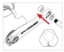
• Tighten the pedals with the recommended torque: 20 – 40Nm (check pedal manufacturer specifications).
