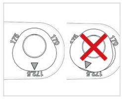
Insert the Tri-lobe nut from the backside. Make sure the holes of the washer and nut are concentric with each other.
