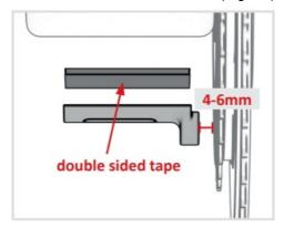
It is recommended to temporarily fix the magnet in place and confirm the correct position before installing with the double-sided tape. Check the functionality of the PowerMeter before gluing the magnet!
