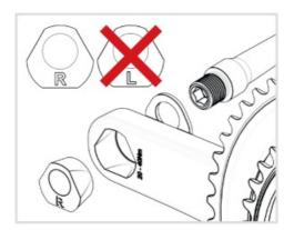
Position the arrow on the Tri-lobe washer facing the marking of the desired length. Make sure the washer is aligned correctly and sitting flush inside the crank (Fig. 4).
