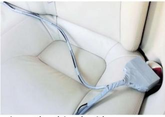
The device with the power wiring is on the driver's side (the device without the power wiring is on the passenger's side)
