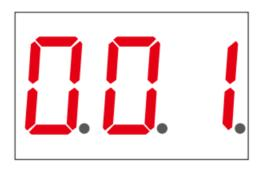
DMX signal indicator (the digit 0 of "hundreds" position of DMX address): When DMX signal input is detected, the digit 0 of "hundreds" position of DMX address will stay solid on. If there is no signal input, the digit 0 of "hundreds" position of DMX address will blink.
