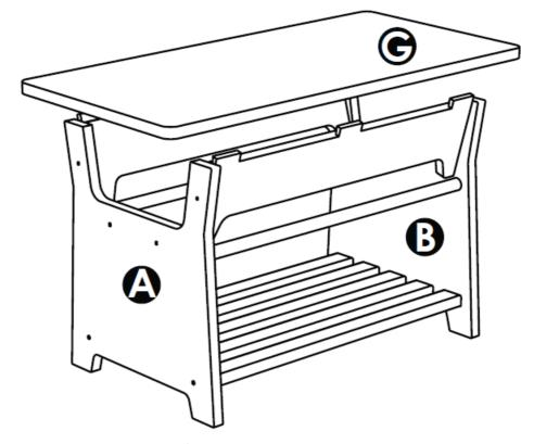
7. Using a rubber mallet, push the Table Top **G** sideways so the tabs lock in with the notch as pictured above.
