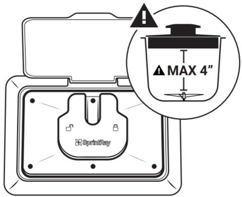
Remove the basket and place the Pro95/S build platform in the wash chamber. If using Pro55/S, use the provided adaptor (see Section 7). Use the touchscreen to select a cleaning cycle.
