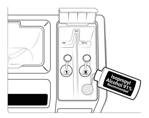
**Minimum** 500 mL Required per tank **Maximum** 2 Liters Required per tank
