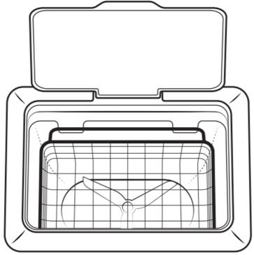
To use the basket, place models inside and close the lid. Use the touchscreen to select a cleaning cycle. The system will not start if the lid is open.
