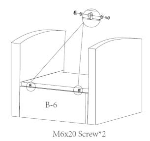
DO NOT tighten any screws before assemble completely .
